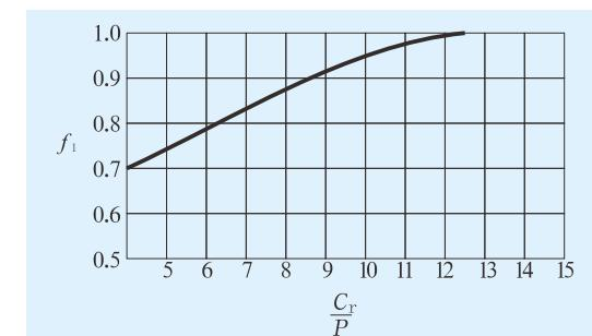
Fig. 10.1 Values of correction coefficient of load condition  $f_1$
