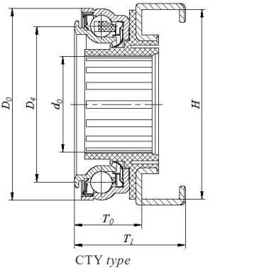
CTY type clutch release bearing unit
