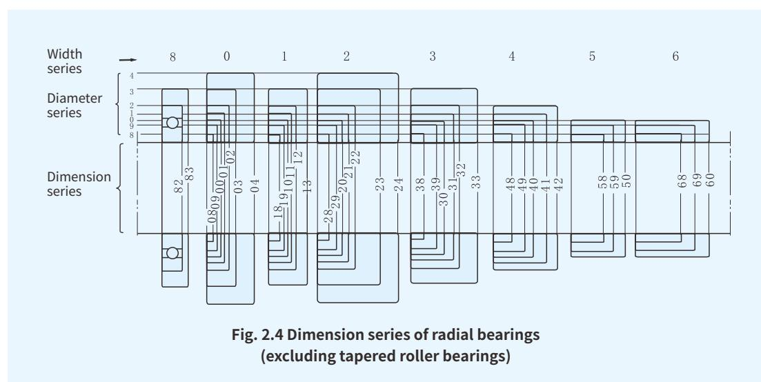
**Fig. 2.4 Dimension series of radial bearings
