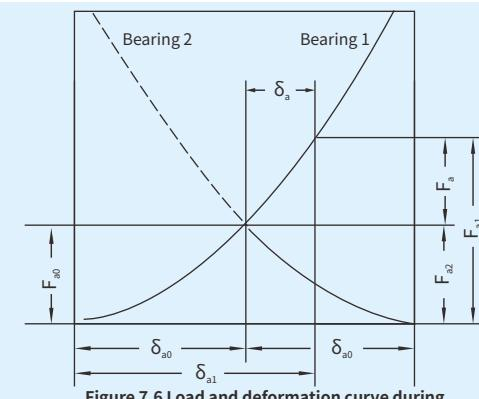
Figure 7.6 Load and deformation curve during constant pressure preload
