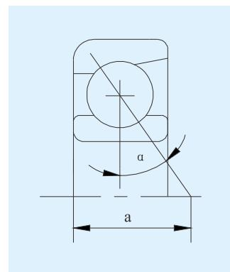
**Table 1 The structures and features of matched pair angular contact ball bearings**
