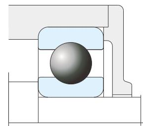
**Fig. 9.2 Non-contact sealing**
