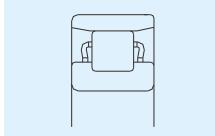
NJ type: outer ring with two ribs, inner ring with single rib
