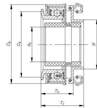
CT/RCT type clutch release bearing unit
