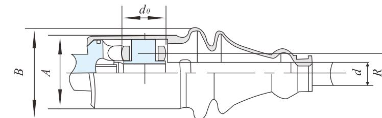
Boundary dimensions of RF type universal joints (Fig as above)
