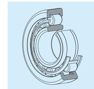
Cylindrical roller bearings mainly support radial loads. Since the rolling body is cylindrical, it has a higher load capacity. The rollers are guided by the inner and outer ring's rib. The inner and outer rings can be installed on the shaft or in the bearing housing with tight fit respectively. If there is no rib, the roller can move freely along the axis.
