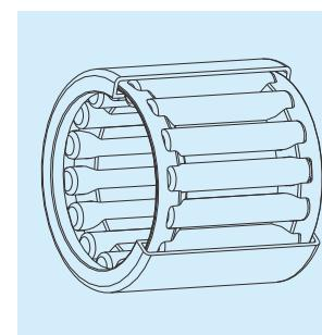
The roller of needle roller bearing is long and thin, with a maximum diameter of 5 mm and a length of 3 to 10 times longer than the diameter. Although the cross-section of needle-roller bearing is narrow, its load is larger than that of ordinary bearings with the same size ratio. Because of the large number of needles, it has large rigidity and small inertia, which is suitable for swinging motion.
