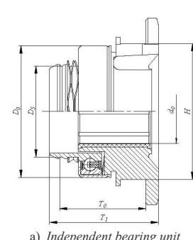
CL type clutch release bearing unit
