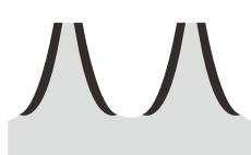
Quenching of gear tooth surface
