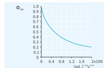
Fig. 2 Coefficient of reduction in cut-in heating Φ<sub>ish</sub>
