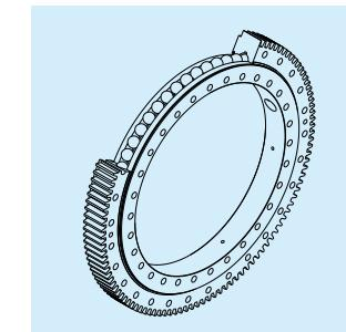
Slewing bearing structure is different from other rolling bearings. It mainly bears axial load and part of radial load, and can also bear large tilting torque. Slewing bearing is divided into single row four-point contact ball type, double row four-point contact ball type, single row cross-roller type, double row cross-roller type, etc.
