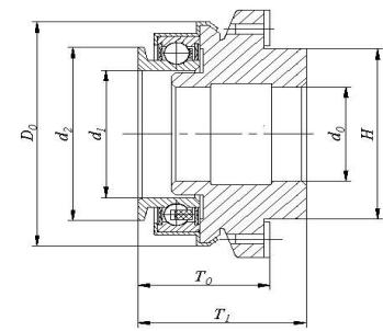
NT/RNT type clutch release bearing unit
