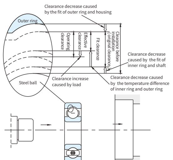
Fig. 6.3 Sketch of single row deep groove ball bearing clearance
