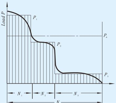
Fig. 11.2 Relations between bearing load and rotation speed
