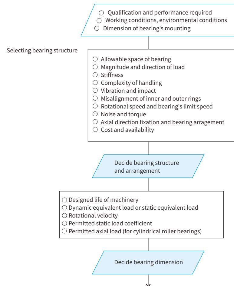
Fig. 3.1 Steps and focus of selecting rolling bearings
