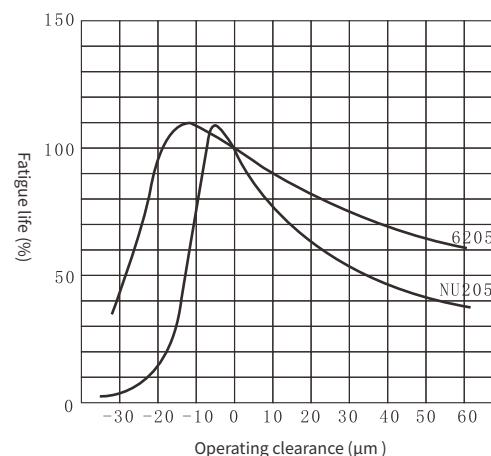
Fig. 6.4 Relation of operating clearance and fatigue life
