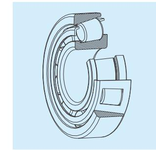
In the design of tapered roller bearings, the conical vertices of the inner and outer rings and the rolling body intersect at the same point on the center line of the bearing. Therefore, the rolling body makes pure rolling motion on the raceway surface, relying on the synthetic force from the raceway of inner and outer ring, and guided by the big rib of inner ring.
