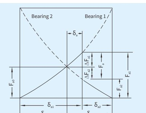
Fig.7.3 Load and deformation curve of angular contact ball bearing during position preload
