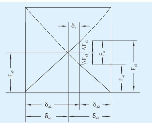
Fig.7.4 Load and deformation curve of tapered roller bearing during position preload
