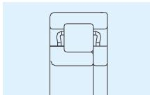
NF type: outer ring with single rib, inner ring with two ribs
