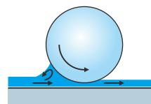
Fig. 1 Lubricant backflow
