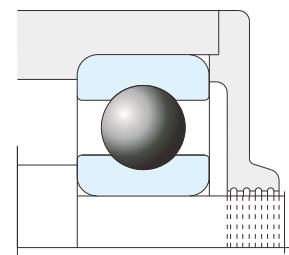
**Fig. 9.3 Concentric oil groove sealing**
