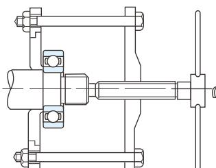
Fig. 12.6 Removal of inner ring using withdrawal tools
