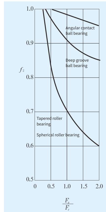
Fig. 10.2 Values of correction coefficient of combined load  $f_2$
