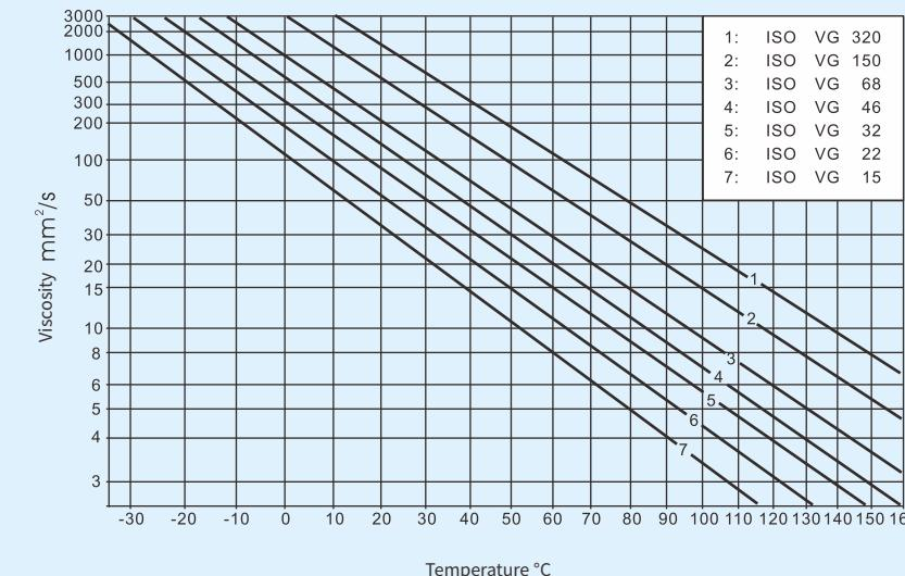
**Fig. 7.9 Corresponding relational graph between lubricating oil viscosity and temperature**
