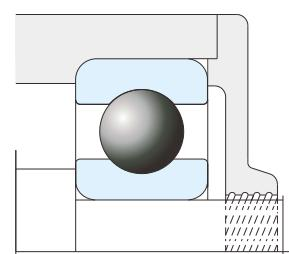
**Fig. 9.4 Spiral oil groove sealing**
