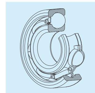
Single row deep groove ball bearings are divided into open deep groove ball bearings, deep groove ball bearings with shields, deep groove ball bearings with seals, deep groove ball bearings with snap rings on the outer ring, etc.
