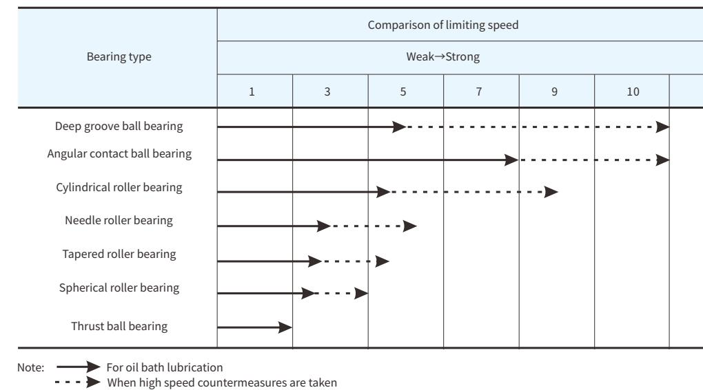
Fig. 4.3 Limiting speed according to bearing types
