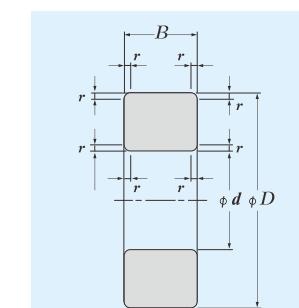
Fig. 2.1 Radial bearing
