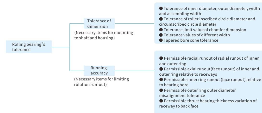
See Table 5.2 for application standards and accuracy class of main bearing types
