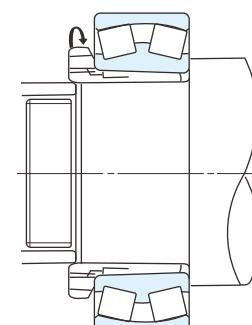
Fig. 12.10 Removal of withdrawal sleeve
