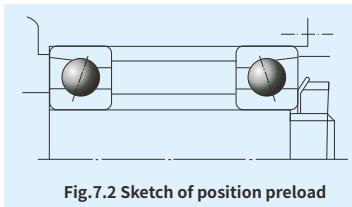
Fig.7.2 Sketch of position preload
