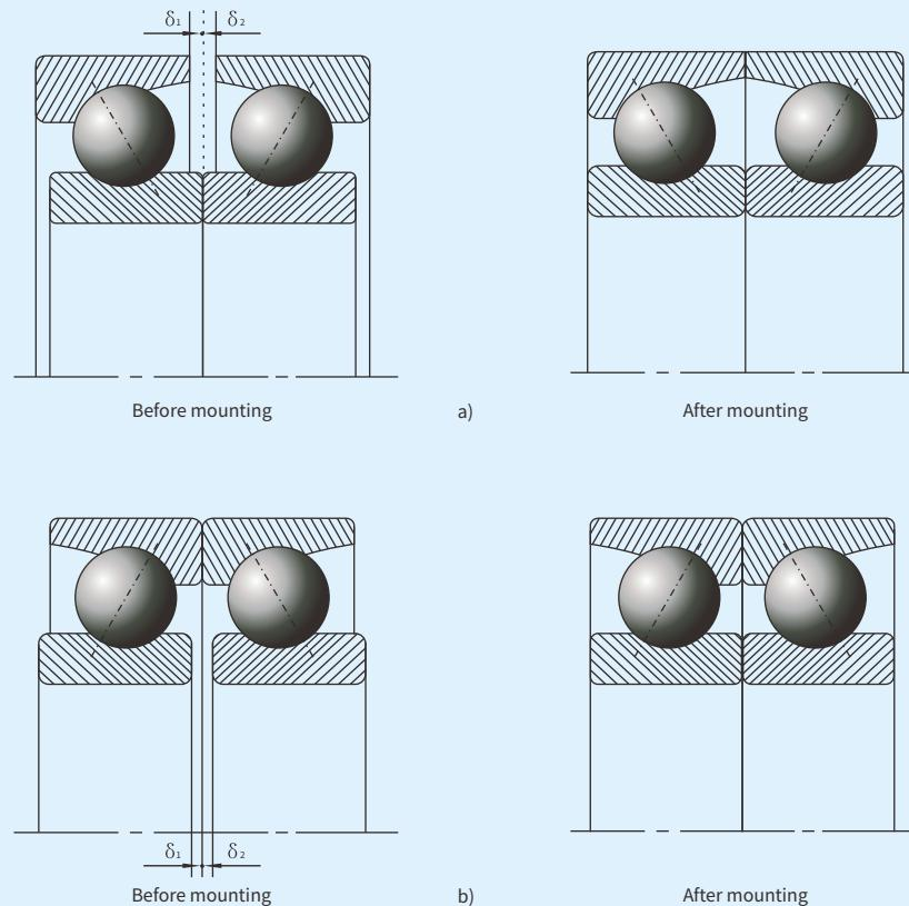
**Figure 7.7 Preload mounting of paired angular contact ball bearing**
