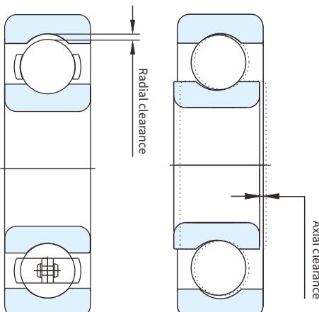
Fig. 6.2 Bearing clearance
