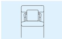
NUP type: outer ring with two ribs, inner ring with single rib and a plate
