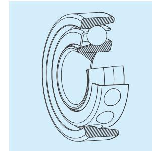
The contact points between the ball and the inner and outer ring form an angle with the radial plane (hereinafter referred to as contact angle). This type of bearing usually has three contact angles: 15°, 25° and 40°.
