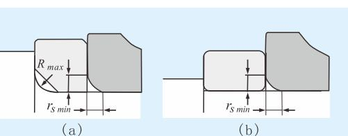
**Fig. 9.1 Bearing mounting with spacers**
