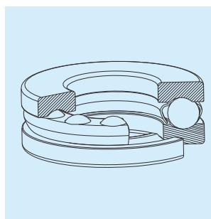
Thrust ball bearings can only bear axial load. This kind of bearing has low rotation speed and special lubrication requirements.
