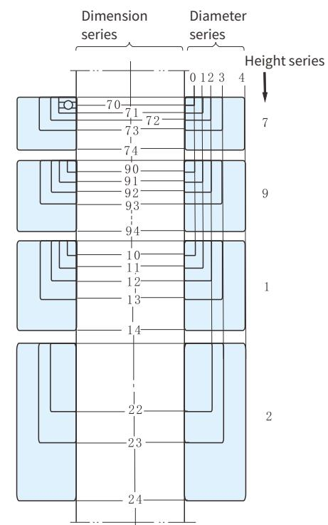
**Fig. 2.5 Dimension series of thrust bearings**
