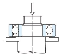
Fig. 12.5 Removal of inner ring using press machine
