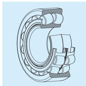
The outer ring of spherical roller bearing is barrel-shaped, with double row inner ring raceway and spherical roller body (also known as drum roller). The center of the outer ring raceway surface coincides with the bearing center, so it has automatic alignment performance. Even if there is installation error or deflection between the shaft and bearing housing, the inner and outer rings can be used when misalignment exists between the bearing rings.
