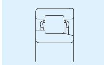
NU type: outer ring with two ribs, inner ring without rib
