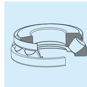
Rollers of this kind of bearing are barrel-shaped. Since the raceway in the housing washer is spherical, the bearing has self-aligning ability. Barrel-shaped roller are arranged diagonally, therefore the deflection of the axle is permitted. Spherical thrust roller bearings have very large axial load bearing capacity, which can bear axial load as well as a certain amount of radial load.
