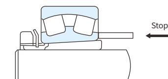
Fig. 12.9 Dismounting bearings with adapter
