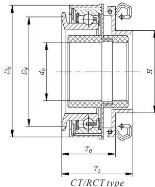
CT/RCT type clutch release bearing unit
