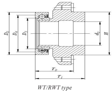
WT/RWT type clutch release bearing unit
