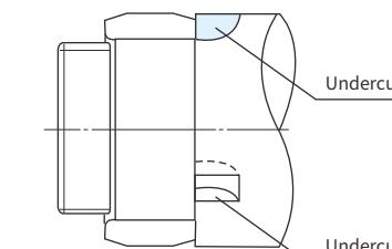
Fig. 12.7 Cut grooves for withdrawal force
