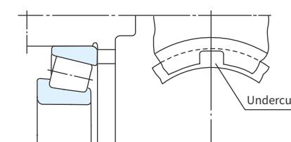
Fig. 12.8 Cut grooves for dismounting outer ring
