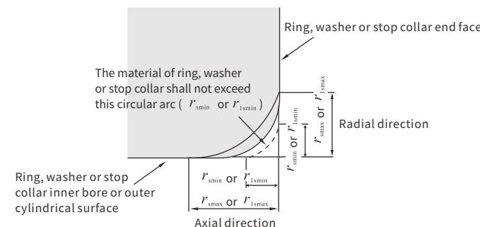
**Table 5.9 Chamfer limit of tapered roller bearing (metric series)**
