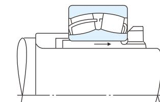
Fig. 12.3 Mounting with adapter
