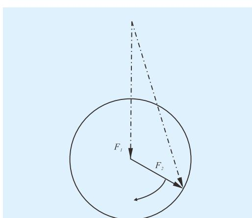
Fig. 11.4 bearing load composed of  $F_1$  and  $F_2$ .
