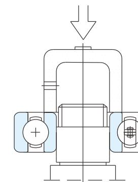
Fig. 12.1 Force mounting of inner ring
