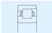
The cages of bearings of the above structures often include: pressed steel, nylon, etc. Some models can be full of rollers without cages.
