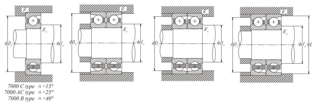
7000 C type  $\alpha = 15^\circ$ 7000 AC type  $\alpha = 25^\circ$ 7000 B type  $\alpha = 40^\circ$
