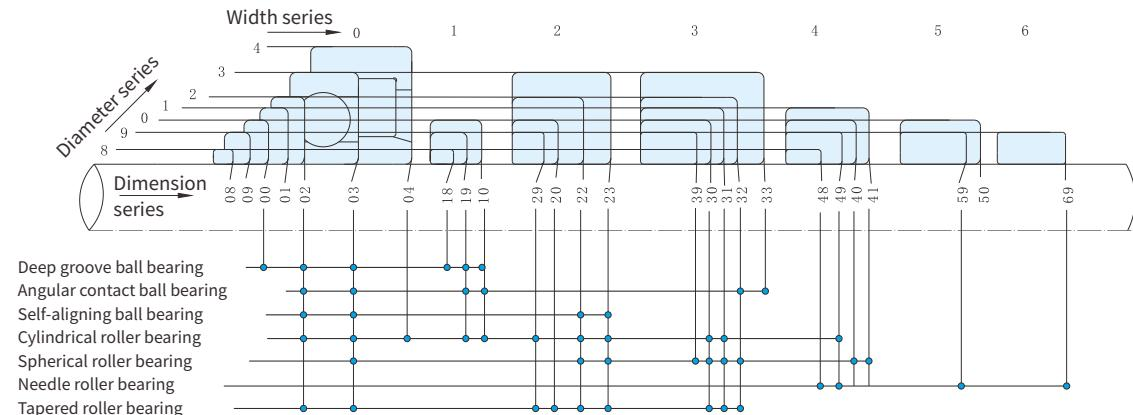
Fig. 4.1 Dimension series and bearing types of radial bearings
