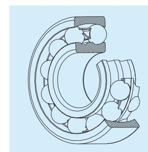
The inner ring of the self-aligning ball bearing has two raceways, and the outer raceway is spherical. The curvature center of the spherical surface coincides with that of the bearing axis. The inner ring, ball and cage can tilt relatively freely to the outer ring. The outer raceway has automatic self-aligning performance.
