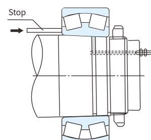
Fig. 12.11 Dismounting using oil pressure
