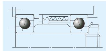
Figure 7.5 Sketch of constant pressure preload
