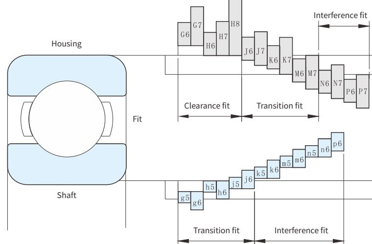
Fig. 6.1 Dimension tolerance and fit of shaft and outer bore
