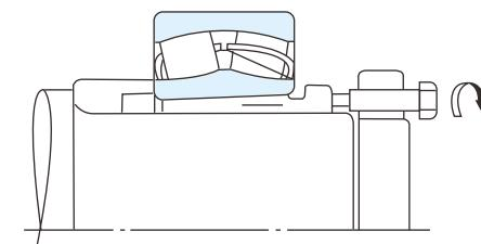
Fig. 12.4 Mounting with withdrawal sleeve
