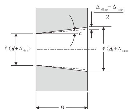
Tapered bore with single plane mean bore diameter deviation
